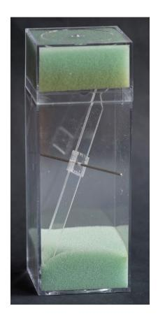
A McMorran Yarn Balance, shown on the left, allows us to calculate the yards per lb. of any yarn. It is well worth the small cost. Follow directions provided with the balance carefully.
