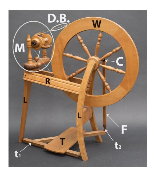
Listed here are the parts of the Scotch tension spinning wheel and their functions; a front view is shown on the left and the back view on the next page; the mother-ofall is described separately with close up views in the following pages. In contrast to other spinning wheels, here the drive wheel rotates the flyer.
